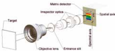
Principle of Spectral Camera
