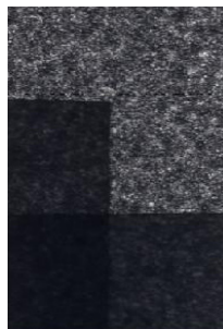
One, two, and three layers of Benadryl™ Quick Dissolve Strips scanned in transmittance.
