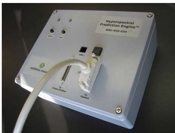
Fig 5 Hyperspectral prediction module. Equations are downloaded into the module and composition prediction is achieved at the speed of the camera for each spatial point.
