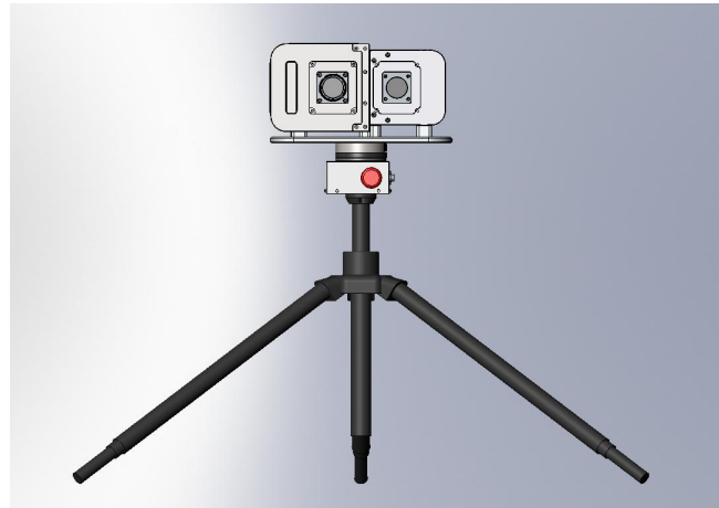
Schematic image of the dual camera setup on a tripod and rotary stage
