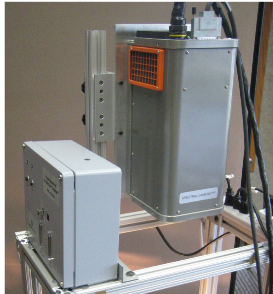
SWIR camera mounted for industrial monitoring
