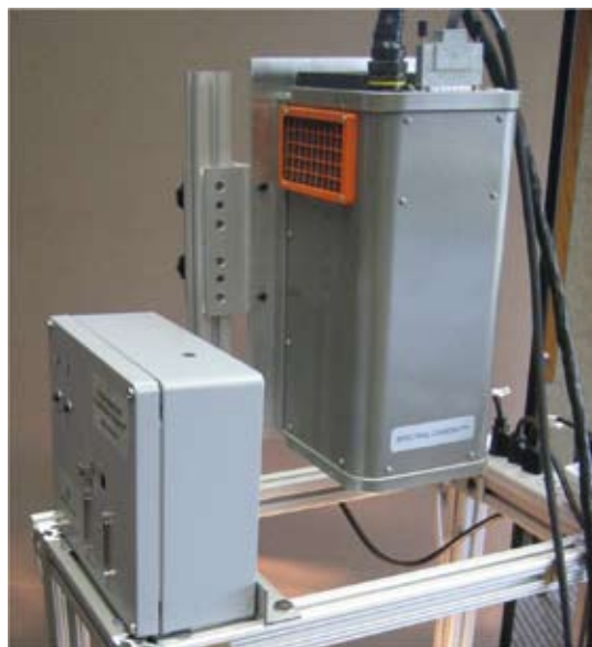
SWIR camera mounted for industrial monitoring
